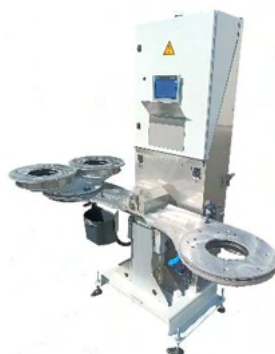
Brazing works flexibility with one or two operators per station, as well as one to four brazing jigs per station.
